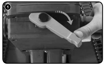
Using the handle position lever (Fig. 1).
