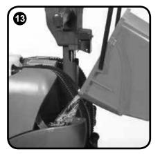
The large cap on the left can be removed for filling from a bucket or suitable container (Fig.13).
