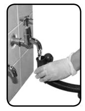
Fill the clean-water tank to a maximum of 40 litres, including cleaning chemicals if required. Follow chemical manufactures guide lines.
